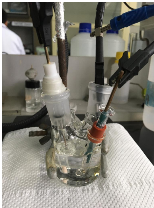
Figure 2.6. Set-up for the cyclic voltammetry. Source: Own elaboration
