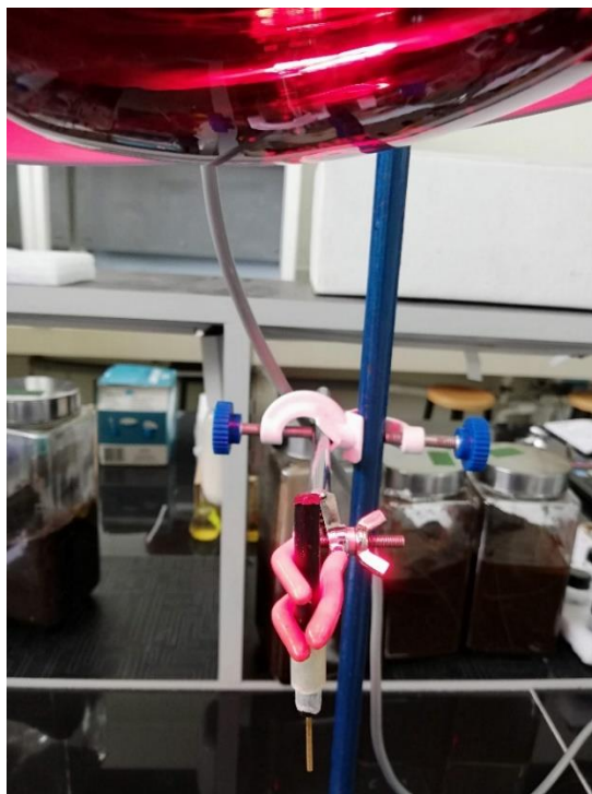
Figure 2.5. Silver nanoparticles ink drying by IR light over buckypaper pasted over carbon vitro work electrode
