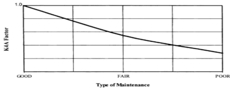
Figure 5.20 K4A = Effect of maintenance on potential idler life.
