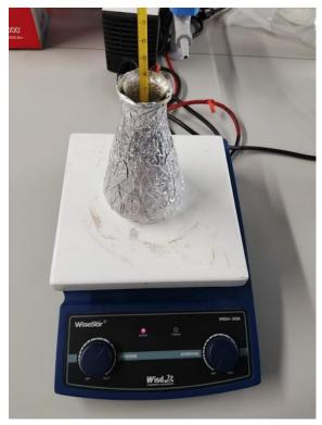
Figure 2.3. Erlenmeyer flask with a magnetic pill totally covered with aluminum foil being heated for the Frens method synthesis of silver nanoparticles.
