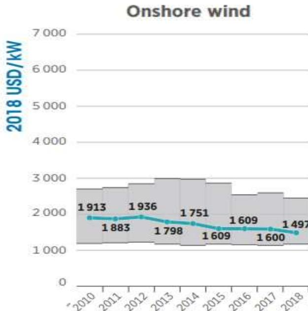
**Figura 2.4** Global weighted average total installed costs for Onshore Wind 2010-2018
