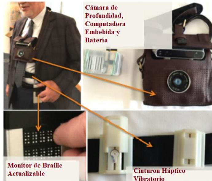
**Figura 1.6.** Wearable Vision-based feedback system.
