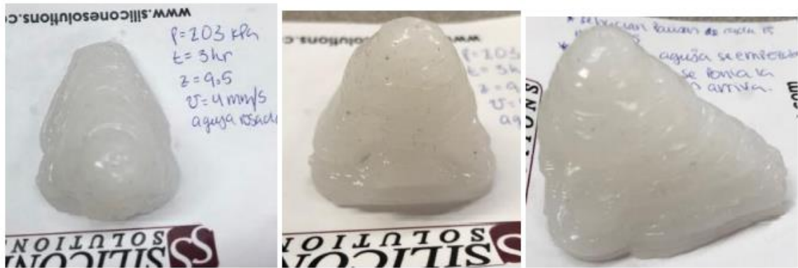
Figure 4.6. Human nose printing using a 20G needle with a pressure of 203 kPa at a speed of 4 mm/s.
