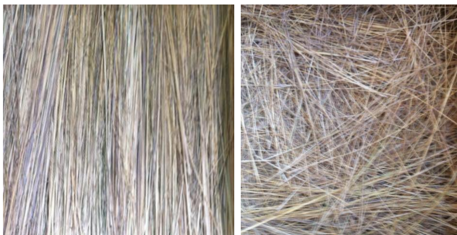
Figure 9: Unidirectional and non-unidirectional non-crushed fiber mat for thermal conductivity measurements
