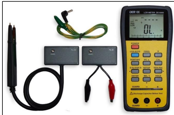
Figure 2.3. RLC-meter IET DE-5000.
