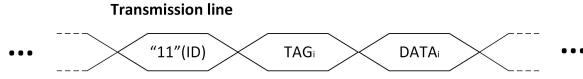
Fig. 2. Timing diagram of the universal link for inputs i from 0 to N . We show the new communication protocol including the initial '11' identifier.
