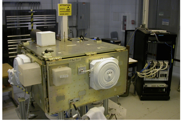
Fig. 14. A spacecraft "concept bus", used to study modularization of plug-and-play spacecraft with integrated wiring, illustrating pegboard panel conventions and a number of mounted components. Equipment rack in background operated test bypass circuitry.
