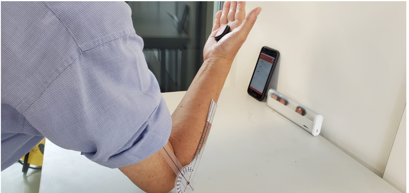
Figure 10. Experimental procedure for angle measurements in two dimensions compared with the angles obtained from the IMU system. The vertical arm of the compass (in white) was fixed onto the lateral side of the upper arm. In contrast, the horizontal arm was mobile to perform accurate 180° amplitude rotations between two segment movements. IMUs and goniometer system coordinates are presented in red and dark grey, respectively. The errors between the two systems are a range of 5% errors.
