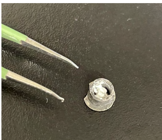
FIGURE 4.14: Nanogel sample loaded into a small inert container specifically designed for thermogravimetric analysis
